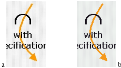
Figure 6 Comparison of quality. a) image compressed with JPEG (arrow has blurred edges); same image compressed with region-based method (edges remain sharp).
