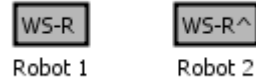
Fig. 15: Two instances of the same template. The model of the instance on the right has been modified after the instantiation; this is denoted by the addition of a marker in the icon.
